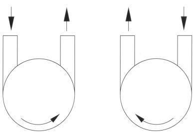
To alter the direction of rotation of a dc motor, reverse the leads. For a single-phase ac motor, reverse the polarity of the start winding in relation to the run winding. If in doubt, obtain the help of a qualified electrician.
